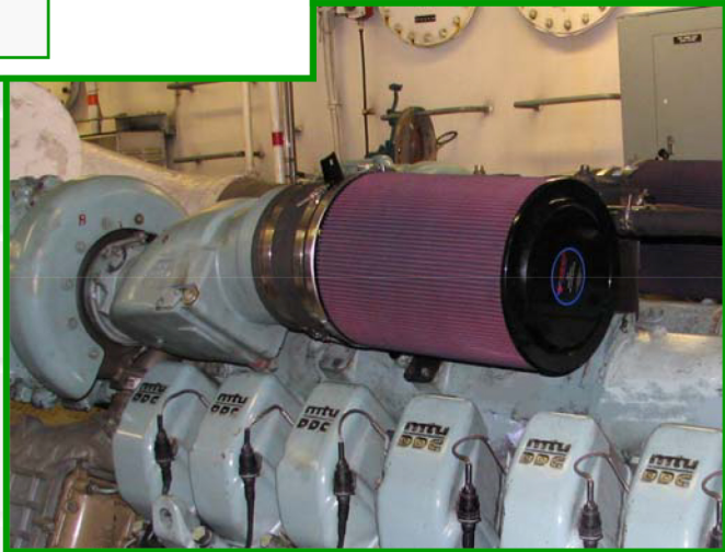
EverQuiet Air Cleaner on a MTU 16V4000.
