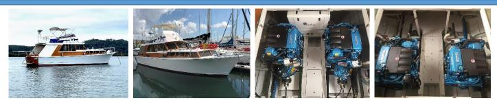
Application: Vessel Name: Vessel Construction: Length (LWL/LOA): Weight: Engine Model: Engine Power: Drive Configuration: Gear Ratio and Model: Gear & Throttle Control Type: Cruise Speed: Top Speed: Propeller Size: Commissioning Date: Halvorsen 42' Viking Balaika Timber 40' / 42' 12 tons T4.230 x 2 plus QMS7.5 Genset 230hp @ 3600rpm Shaft – Down Angle ZF 63A @ 2.04:1 Morse Mechanical 8.5 knots 18 knots 4 Blade, 20" dia x 17.5" pitch 25/07/19
