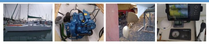
Application: Vessel Name: Vessel Construction: Length (LWL/LOA): Weight: Engine Model: Engine Power: Drive Configuration: Gear Ratio and Model: Gear & Throttle Control Type: Cruise Speed: Top Speed: Propeller Size: Commissioning Date: Sailing Catamaran Mistweaver GRP Composite 39' / 40' 6 tons 2 x N3.21 21hp @ 3600rpm Conventional shaft 2.6:1 TMC40 Morse mechanical 7 knots 9 knots 2 Blade Folding 15" dia x 11" pitch 20/08/20
