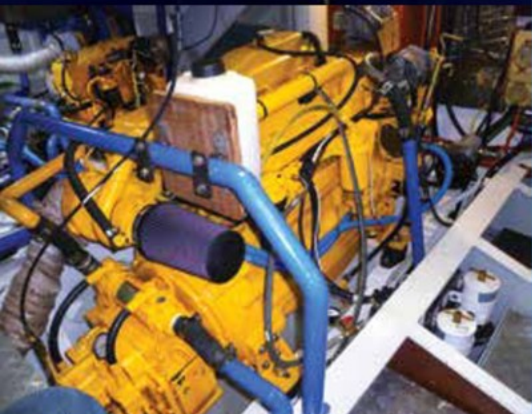
Ken Petch installed the PowerTech 6.8L engine himself, with expert support from Steve Shale at Marine Diesel Pty. Ltd.
