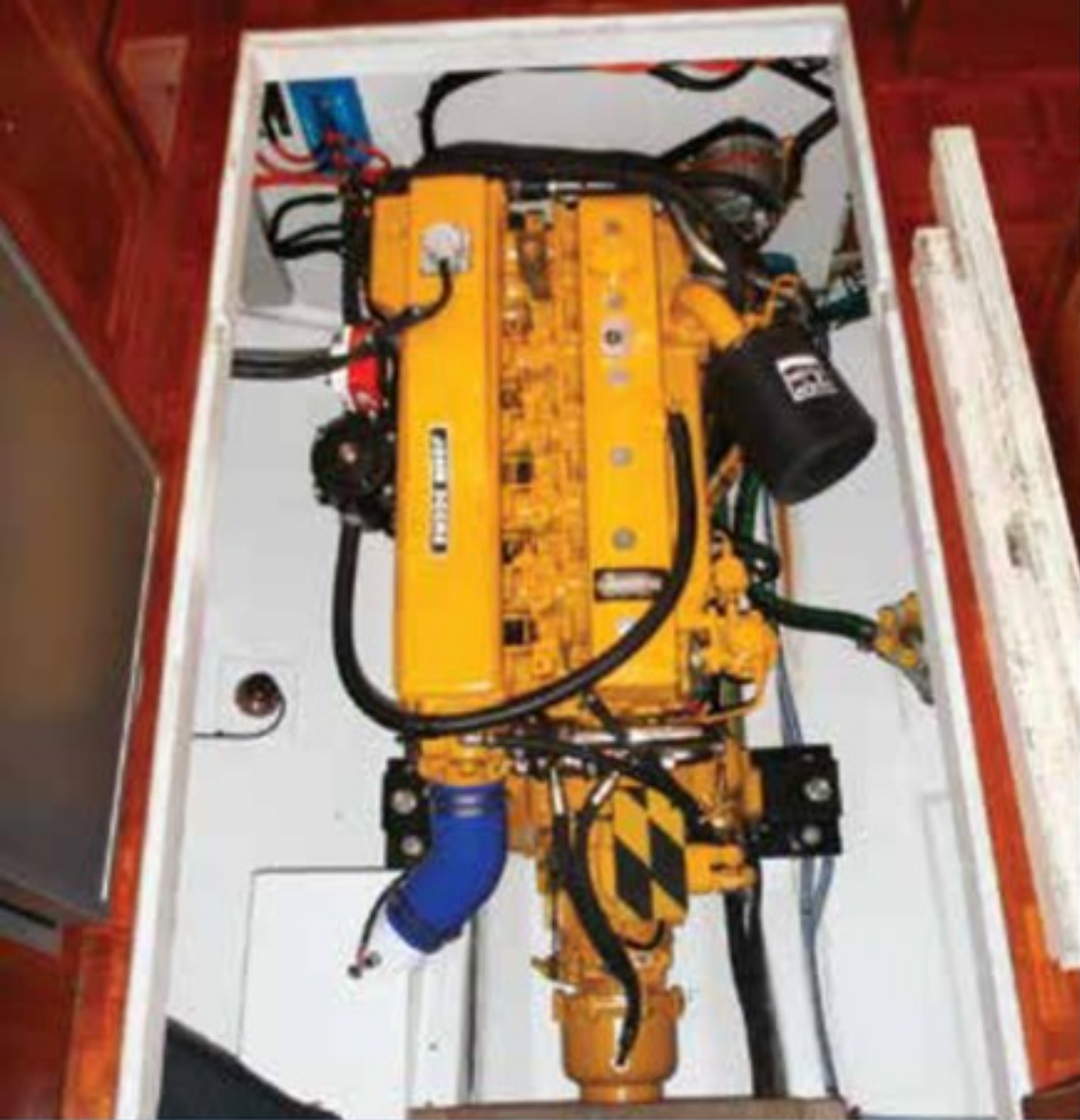
Robert Burton selected the PowerTech 6.8L engine because it offered the right combination of dimensions and power.
